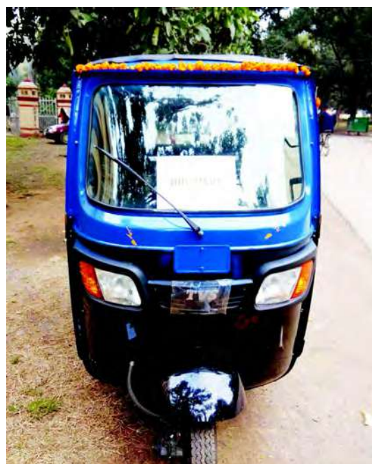
Fig. 17: Hydrogen-fuelled three-wheeler developed at HEC-BHU
