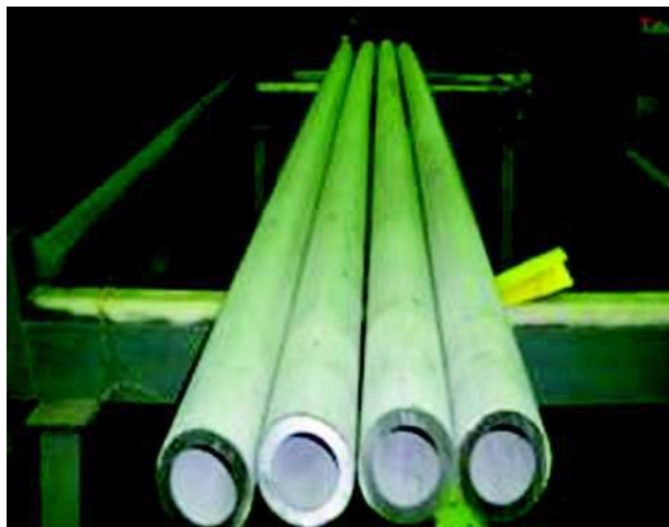
Fig. 4: Indigenously manufactured 304HCu SS boiler tubes of 6-7 m length (Jayakumar et al. , 2014)
