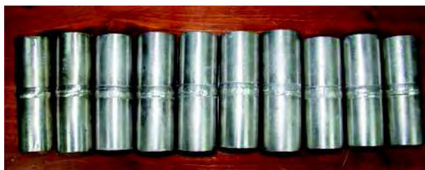
Fig. 5: Welded boiler tubes of indigenous 304HCu SS (Jayakumar et al. , 2014)
