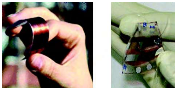
Fig. 13: (A) OSC printed on paper at Chemnitz University of Technology, Germany (Hübler et al. , 2011); (B) OSC fabricated on flexible polyethylene terephthalate (PET) at IIT Kanpur (Dembla, 2009)
