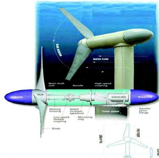
Fig. 4: Tidal turbine configuration. Source: http://www.verdantpower.com
