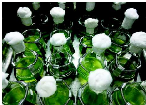
Fig. 4: Cultivation of algae in shake-flasks
