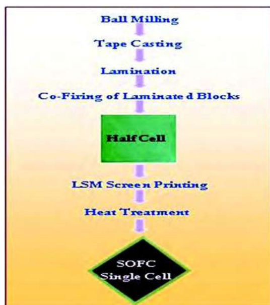
Fig. 23: Flow chart of the single cell fabrication (Basu et al. , 2008)
